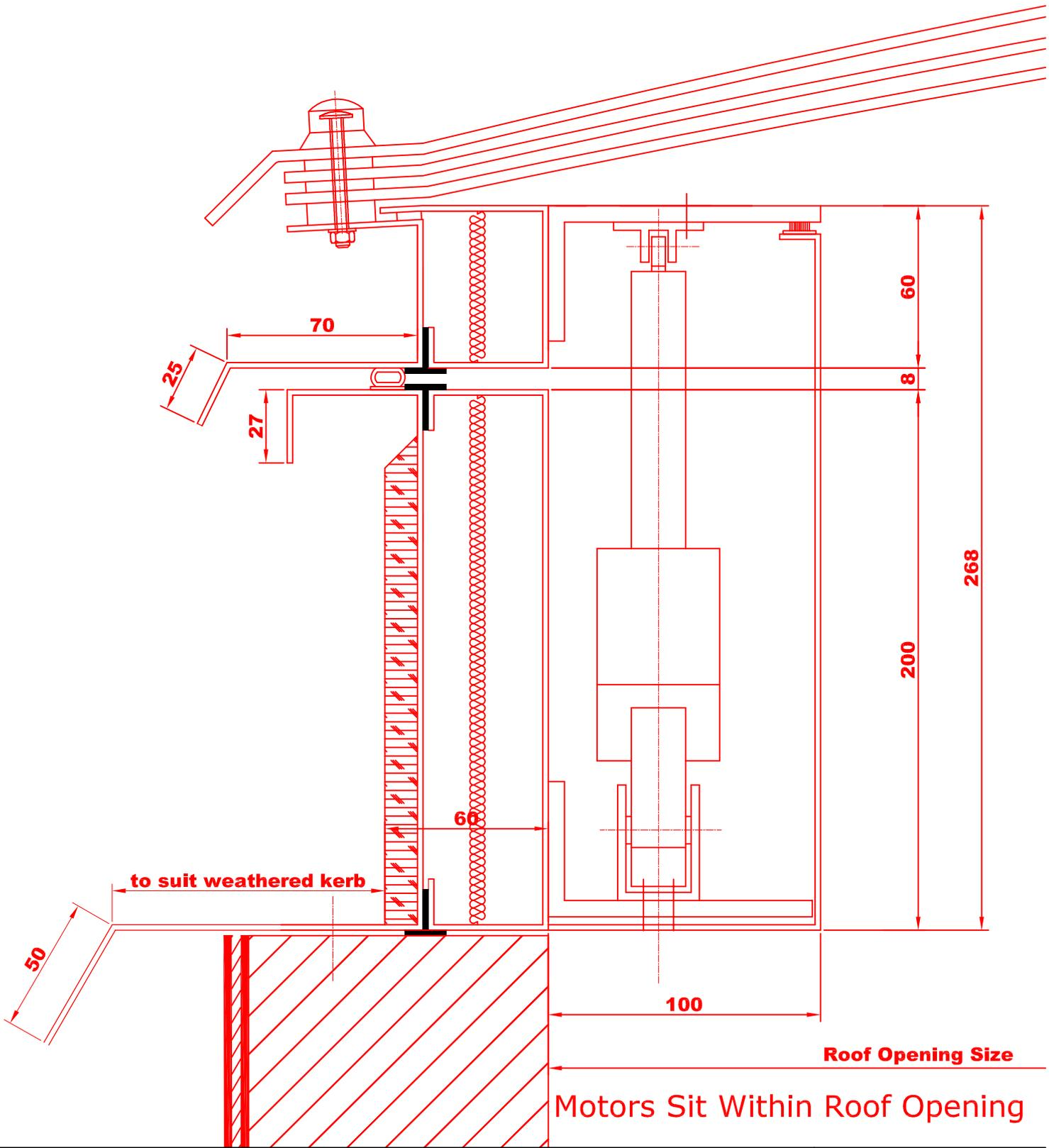
**METAL KERB DETAIL / FAIL SAFE OPENING**
