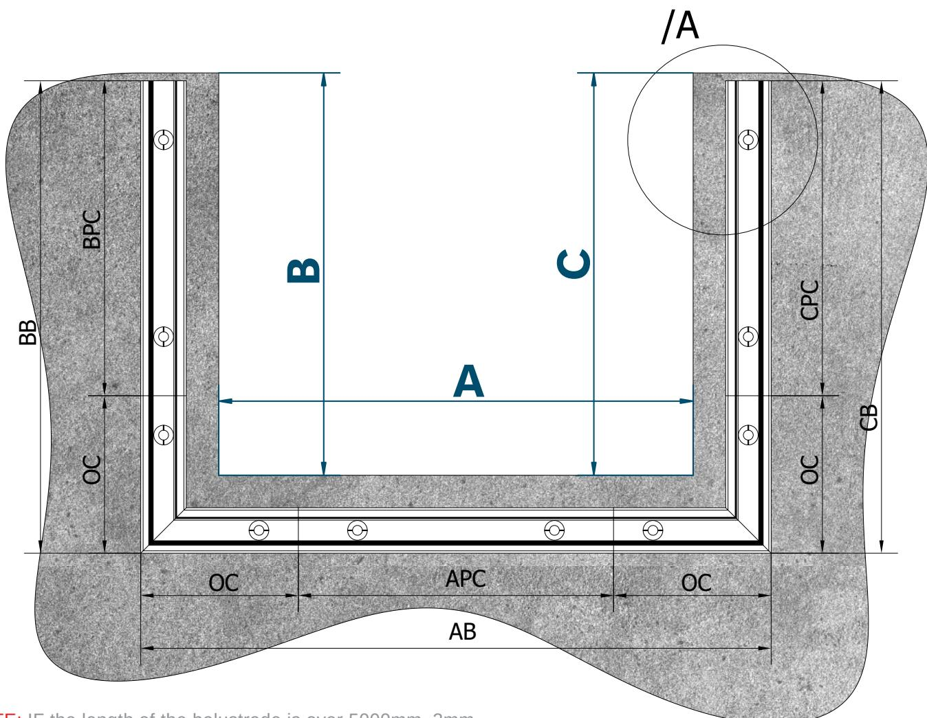
**NOTE:** IF the length of the balustrade is over 5000mm. 3mm thermal expansion joint must be anticipated for every next piece!
