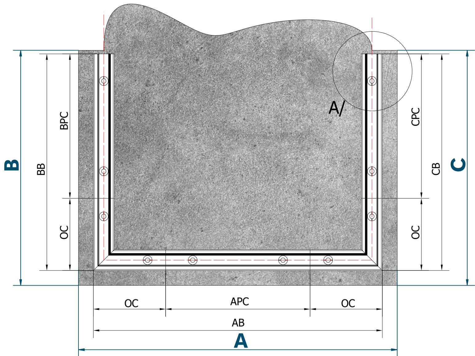
**NOTE:** IF the length of the balustrade is over 5000mm. 3mm thermal expansion joint must be anticipated for every next piece!
