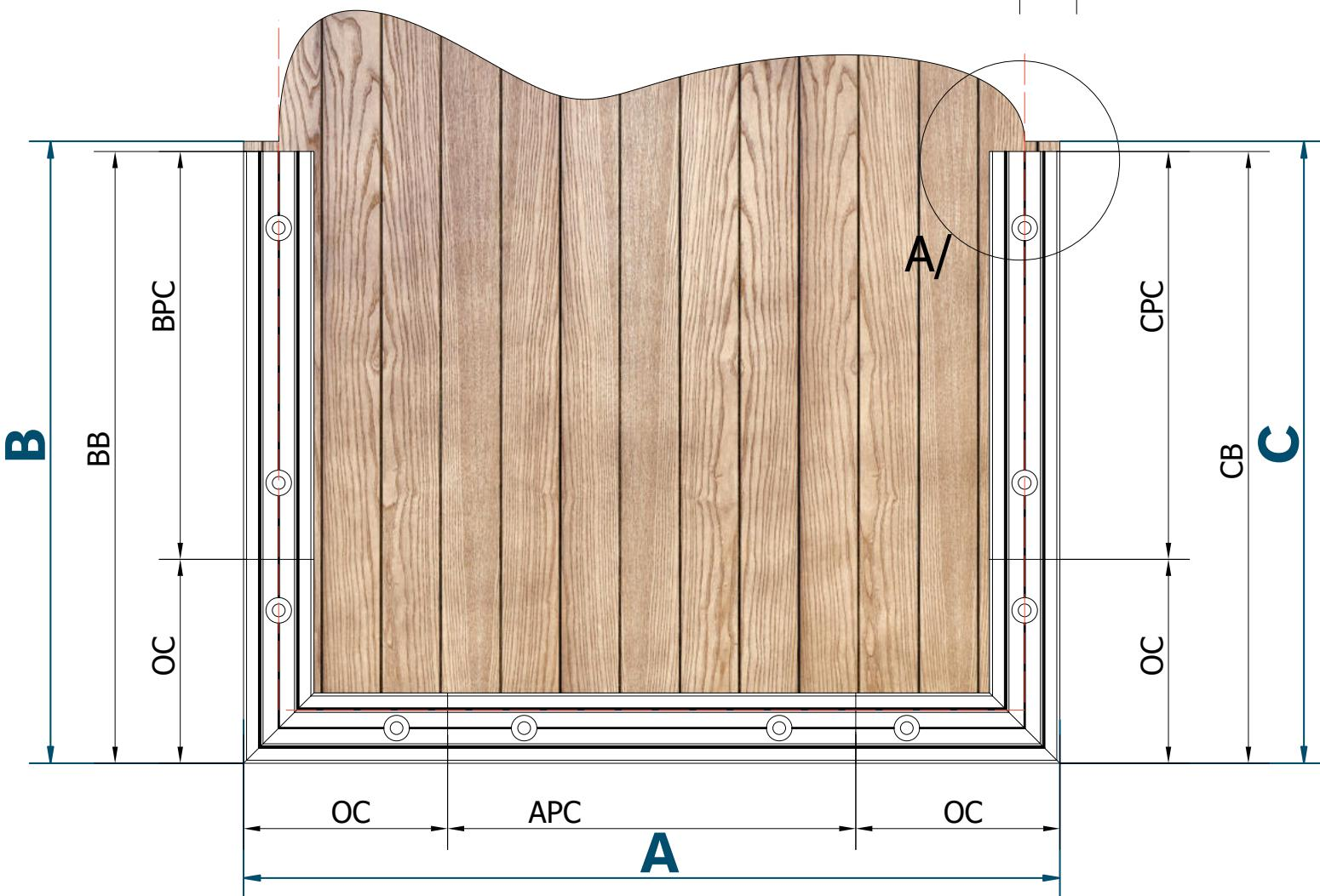
NOTE: IF the length of the balustrade is over 5000mm. 3mm thermal expansion joint must be anticipated for every next piece!
