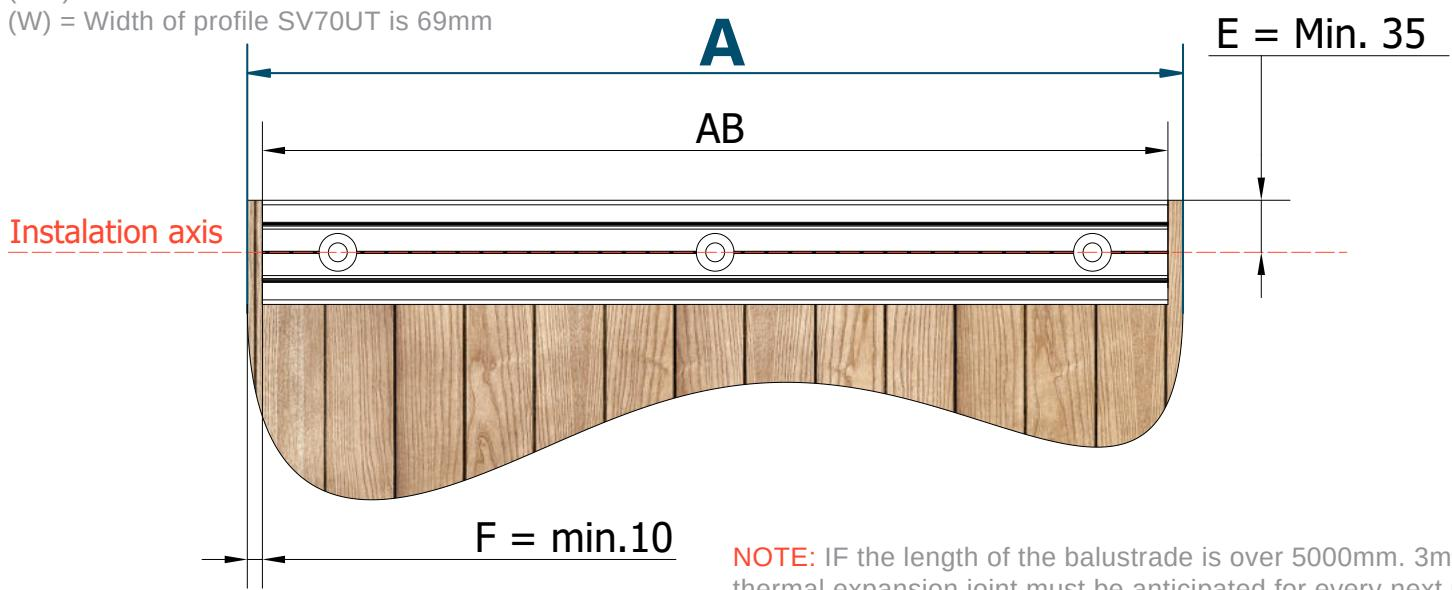
**NOTE:** IF the length of the balustrade is over 5000mm. 3mm thermal expansion joint must be anticipated for every next piece!
