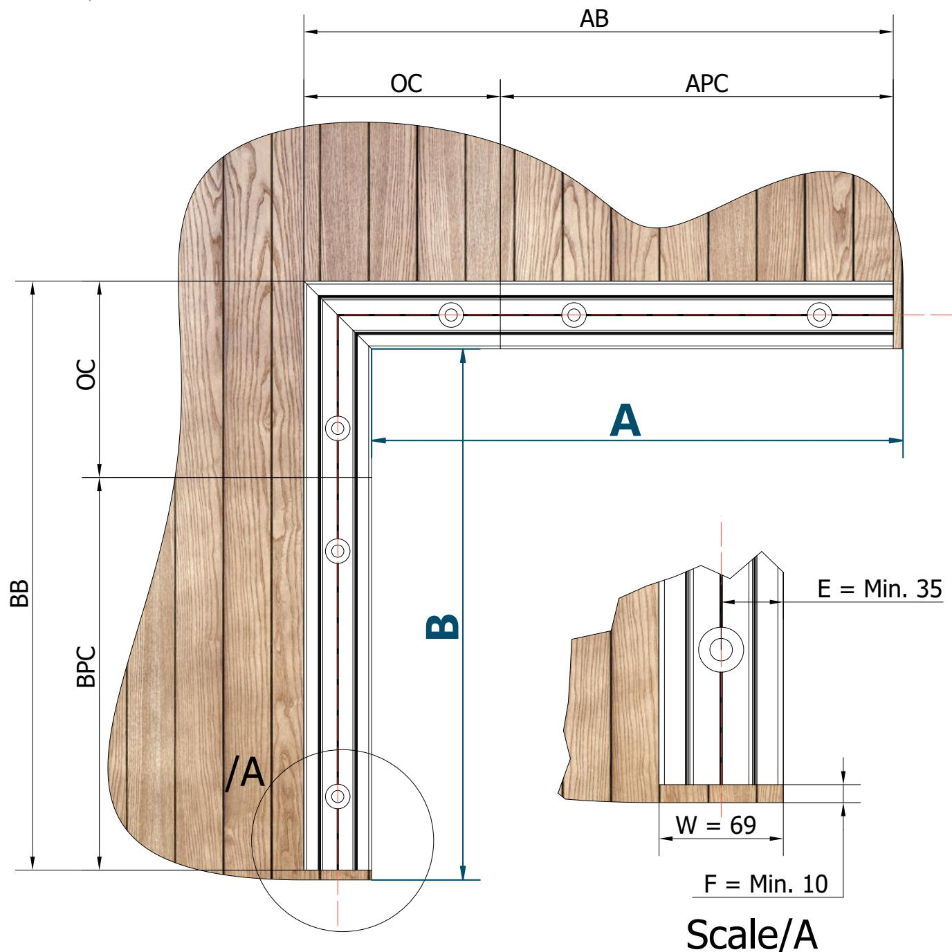
**NOTE:** IF the length of the balustrade is over 5000mm. 3mm thermal expansion joint must be anticipated for every next piece!
