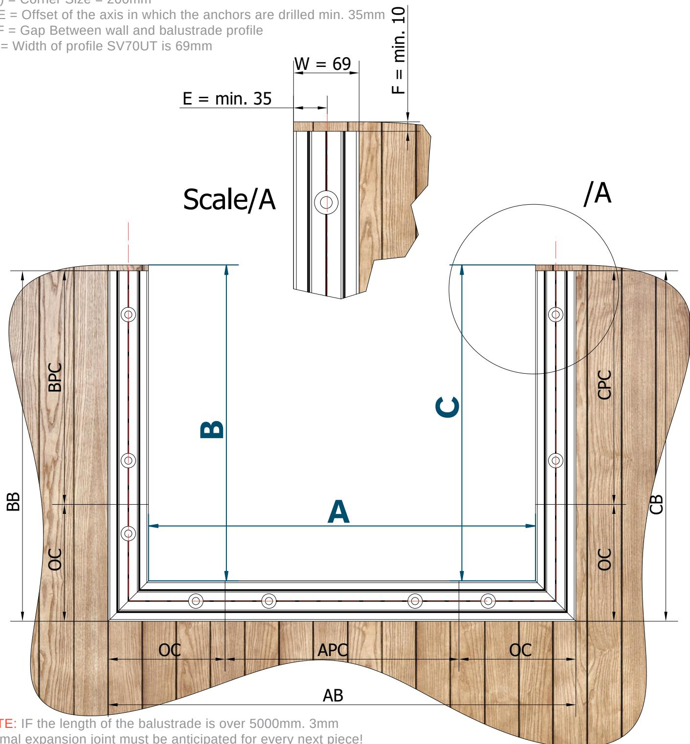
**NOTE:** IF the length of the balustrade is over 5000mm. 3mm thermal expansion joint must be anticipated for every next piece!
