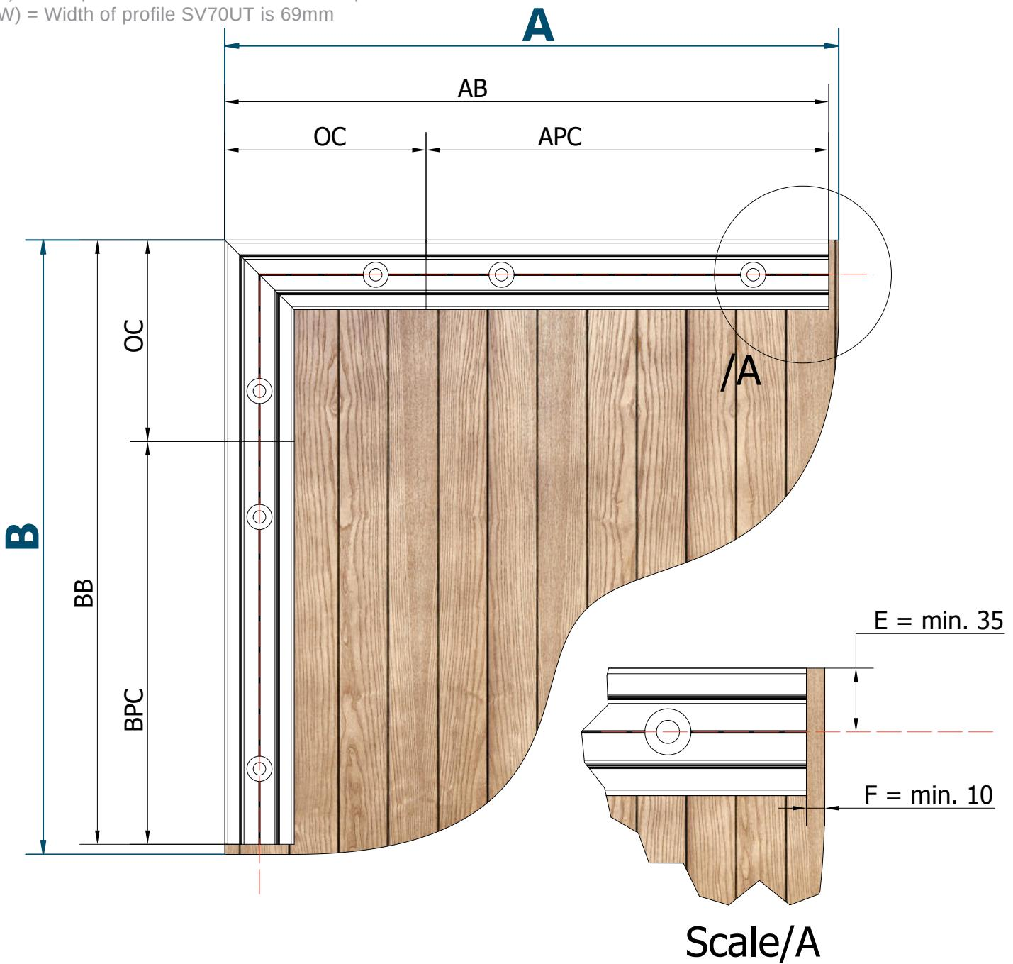
**NOTE:** IF the length of the balustrade is over 5000mm. 3mm thermal expansion joint must be anticipated for every next piece!
