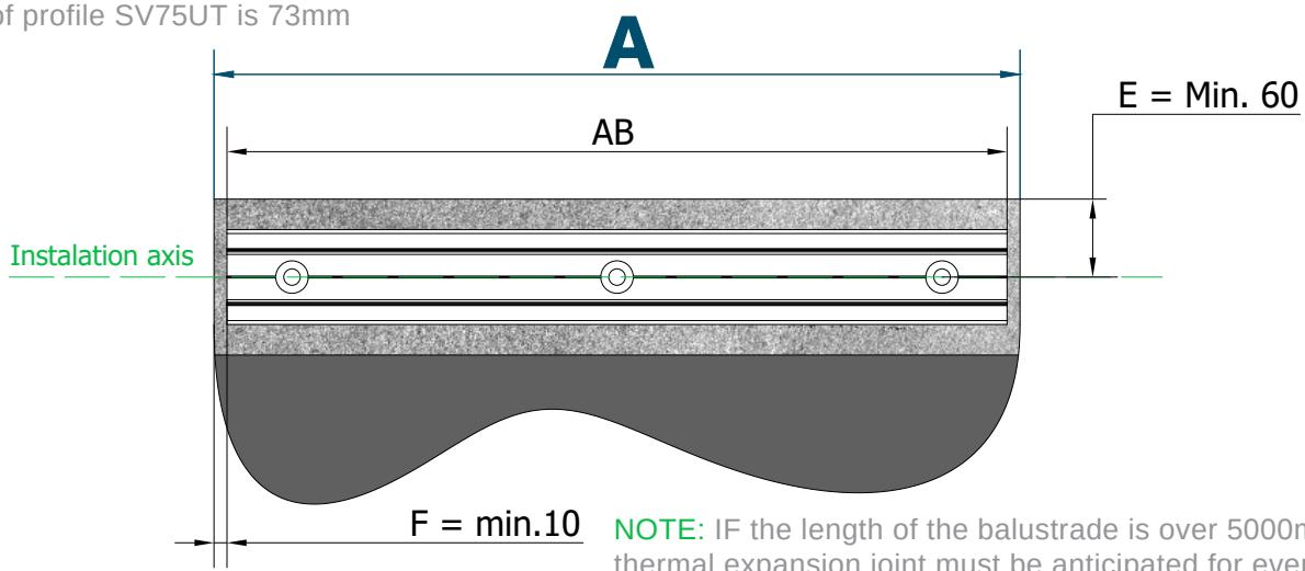
**NOTE:** IF the length of the balustrade is over 5000mm. 3mm thermal expansion joint must be anticipated for every next piece!
