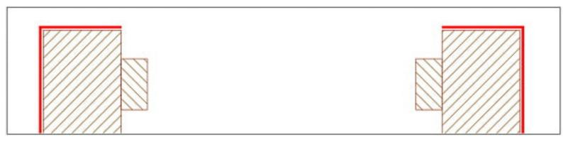
Once you finish weathering the upstand, you are ready to install the Skylight. Make sure all surfaces where the silicone will be applied are clean of dirt, dust, moisture, etc.
