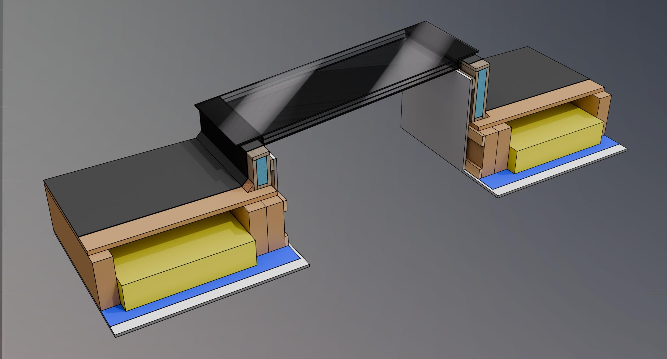
A"cold roof" is a roof design where the insulation sits between the rafters, so the rafters remain uninsulated and act as a thermal bridge/weak point.
