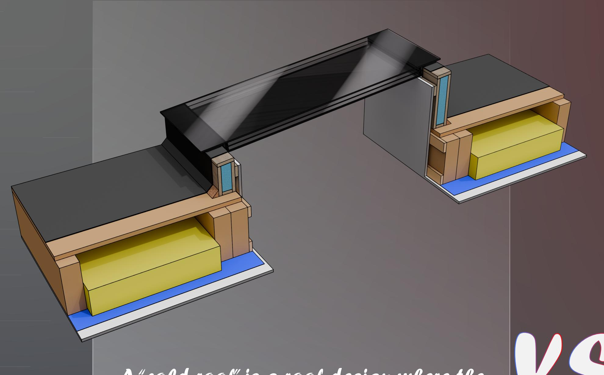
A"cold roof" is a roof design where the insulation sits between the rafters, so
